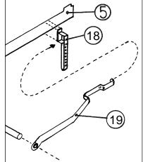
Dress the cusp off the brake levers (parts 19) to make them look a little more delicate. Then form up (note etched dots to mark the position of the handle folds), thread handle through pin guide and solder at vee hanger and pin guide. Cut excess off ends of 1.6mm brass rod and file ends square.
