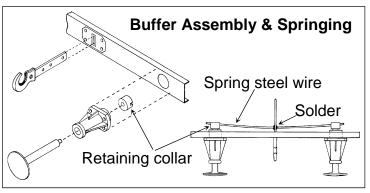
will help prevent the drill wandering in the white metal and breaking through the side of the buffer. Then fit shank through buffer body, snip off some of the narrow end of the shank to leave just over 1mm from the step and solder a retaining collar onto the shank. Fit the cast vacuum brake pipes
