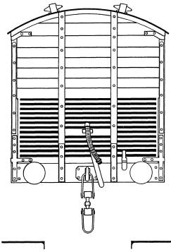
LNER Livery. Bodywork including solebars and headstocks, Red Oxide. Roof, white later grey. Running gear and buffers, black. Lettering, white, pre 1936 as drawing. Post 1936 the 'NE' was reduced to 4", placed over '12T' in 3" which in turn was above the running number in 4". All to the bottom L/H corner with 3" spaces between lines.
