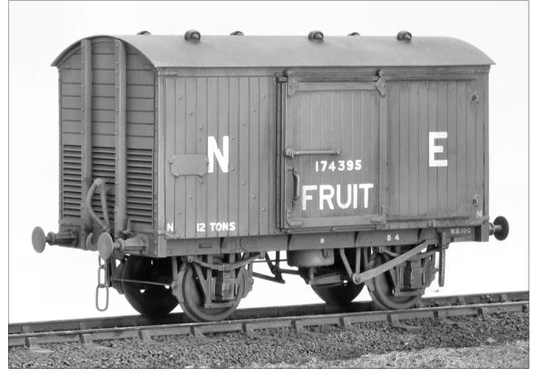
**PROTOTYPE.** These 10ft wheelbase, wooden underframe vacuum braked ventilated vans were built in large numbers during the 1930's. They lasted well into BR days and were used throughout the LNER system to destinations all over Britain.
